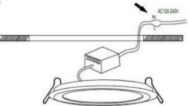
2- connect with the driver, make the insulation measure;
