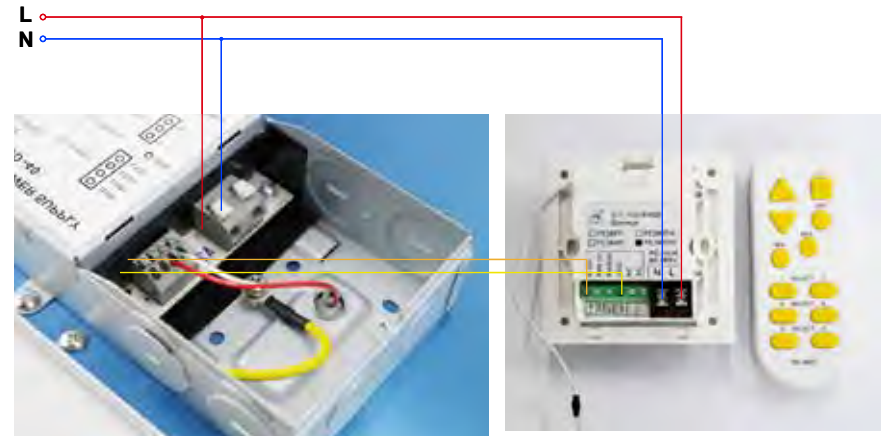
Wiring of panel light with Far infrared remote control dimmer
